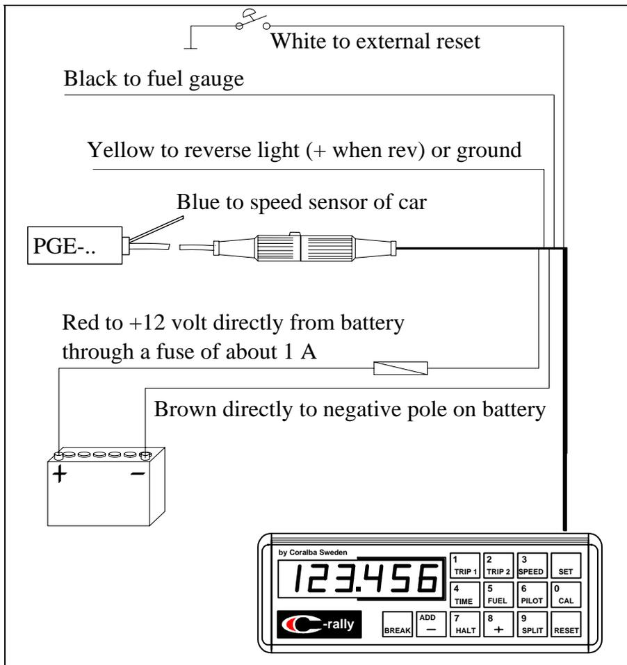
Make sure all connections are done professionally. The cables should be fixed to avoid damage. Most disturbances in function that occur are caused by poor connections to the power supply. After having carried out these functions simply connect each part together and you will be ready to use C-rally.
