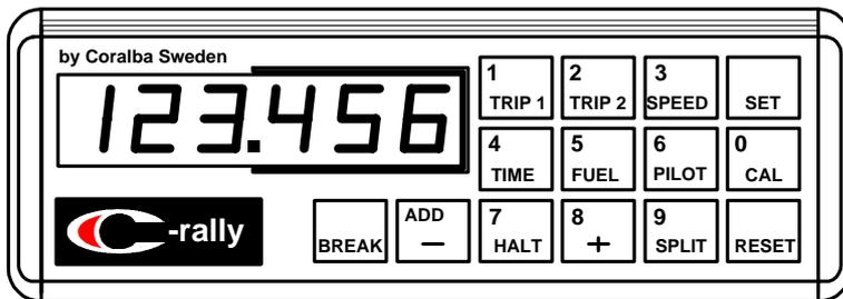
It is basically a distance- and speedo-meter for the car. Furthermore it has a lot of useful processing facilities for the co-driver. The precision of the instrument is reached by an effective but simple calibrating procedure. After calibration C-rally shows correct values to a tolerance typically better than 0.03%.
